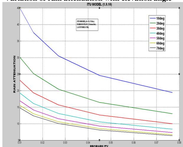
Tabular Form Showing Variation Of Rain Attenuation With Elevation Angle And Probability Of Period Of Reference On 01.09.2010 :
